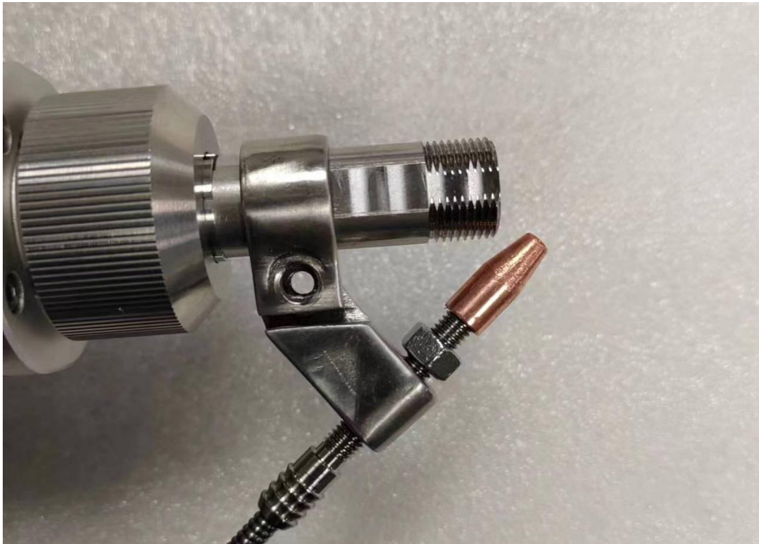
Step 3: Reinstall the copper nozzle tip and adjust the wire feed guide nozzle to a proper position
