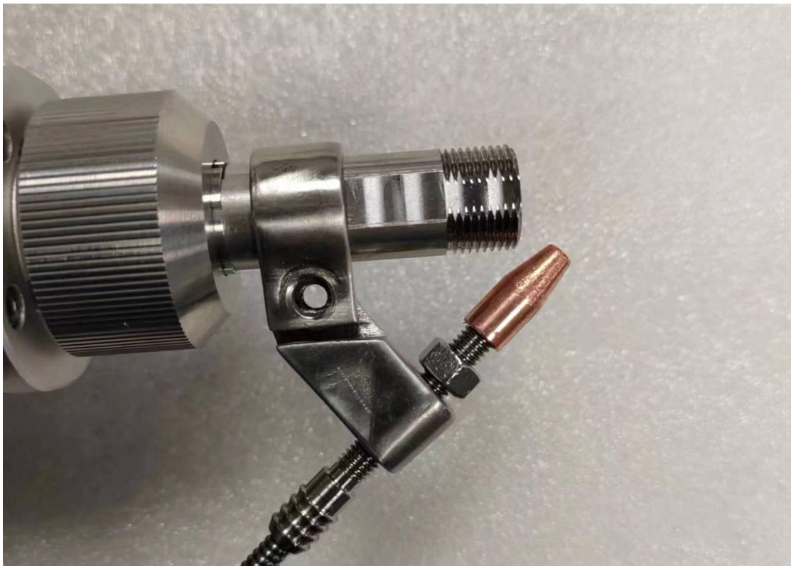
Step 3: Reinstall the copper nozzle tip and adjust the wire feed guide nozzle to a proper position
